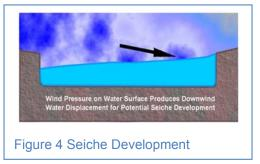
However, during severe storm conditions, water-level differences greater than 5 metres (16 feet) have been observed between opposing lakeshores.
